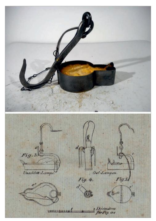
Fig. 8. Iron mine lamp used in late 19th century Austria: top, preserved specimen; bottom, patent drawings (Top, © miners-lamps.com; bottom, after Hartmann 1822: Pl. 1 © e-rara.ch)
